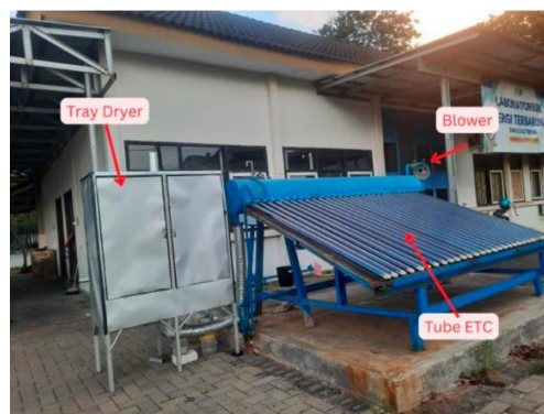
Gambar 1. Sistem ETC solar dryer .
