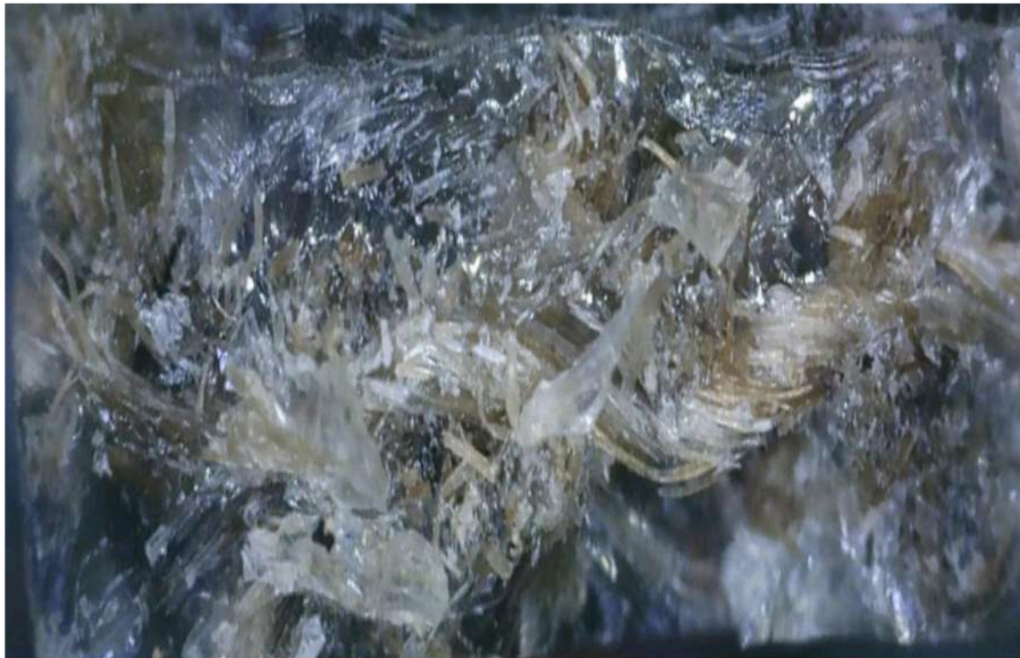
Figure 5. Macro Photograph of Ramie Fiber Reinforced Composite with Alkali Treatment of NaOH 10% and Vacuum Pressure 6 N/mm 2
