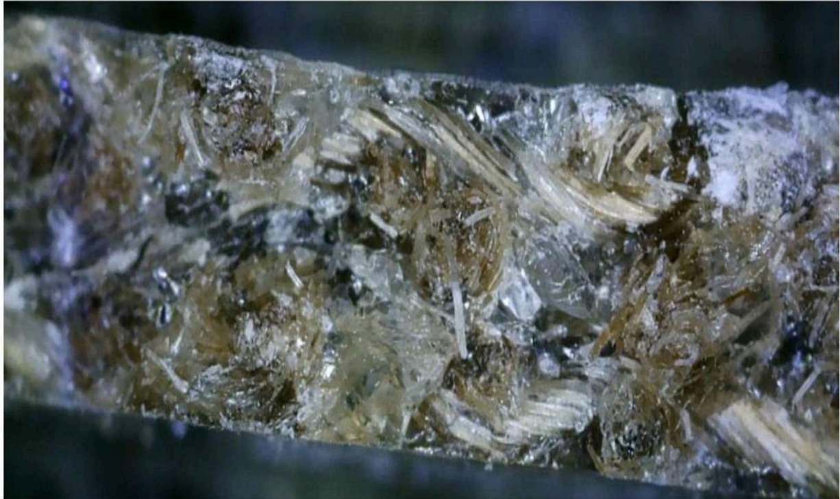
Figure 3. Macro Photograph of Ramie Fiber Reinforced Composite with Alkali Treatment of NaOH 5% and Vacuum Pressure 6 N/mm 2
