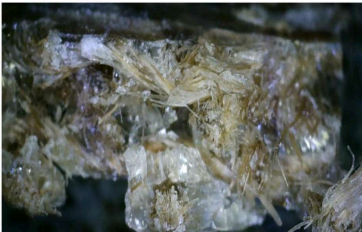
Figure 6. Macro Photograph of Ramie Fiber Reinforced Composite with Alkali Treatment of NaOH 10% Vacuum Pressure 14 N/mm 2
