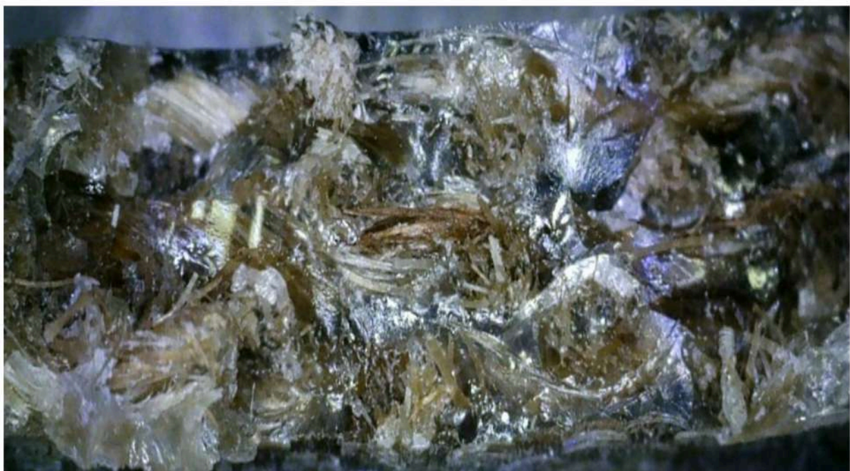
Figure 4. Macro Photograph of Ramie Fiber Reinforced Composite with Alkali Treatment of NaOH 5% Vacuum Pressure 14 N/mm 2
