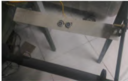
Figure 9: Position of the Ultrasonic sensor.
